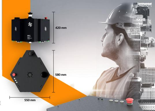
**BRIT** is a stand-alone device that processes CAD files, compares them with the surroundings and prints the information on the ground. In this way, the execution time of a conventional stakeout is reduced with millimetric precision.
